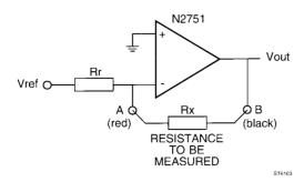
Figure 3.13 Ohm measurement circuitry (principle of operation)
